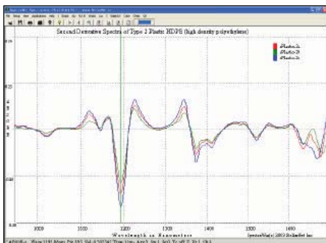
Spectrum from DWARF-Star-512 showing 2 nd Derivative spectral reflectance of type-2 plastics
